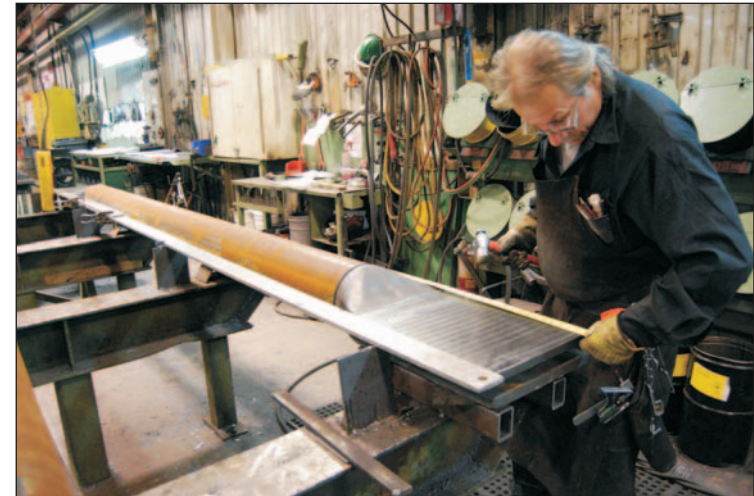
Figure 8: Fitting of HSC brace assembly. Fitter simultaneously ensures:
