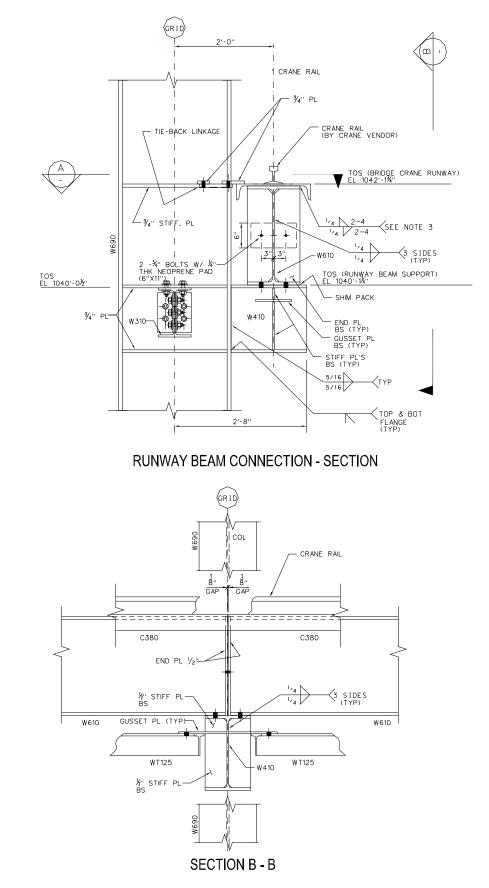
Top Running & Underhung Bridge Crane Crane Load & Crane Runway Beam Design
