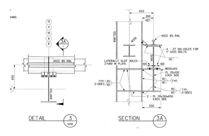
Crane Runway Beam Connection Runway Beam Size W610x155 + PL457x19
