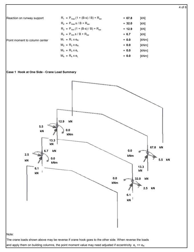
Top Running & Underhung Bridge Crane Crane Load & Crane Runway Beam Design
