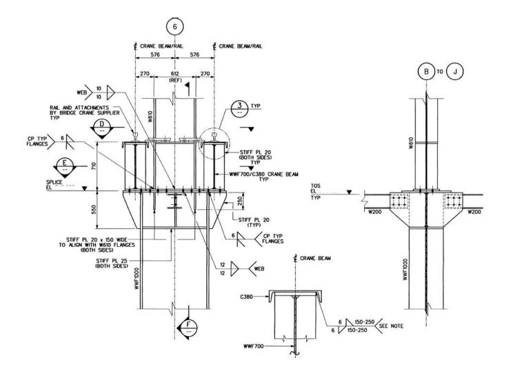
Crane Runway Beam Connection Runway Beam Size Change to W690x125 + C380x50
