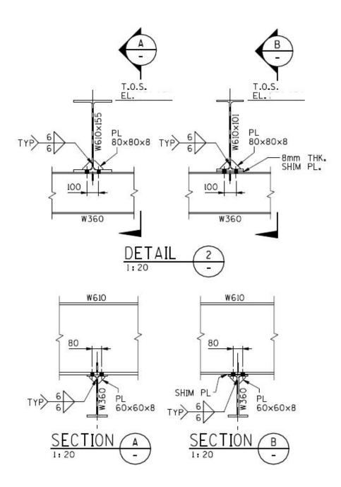
7.5 Tonne Underhung Crane W360x57 Runway Beam Support Point to Floor Beam Connection
