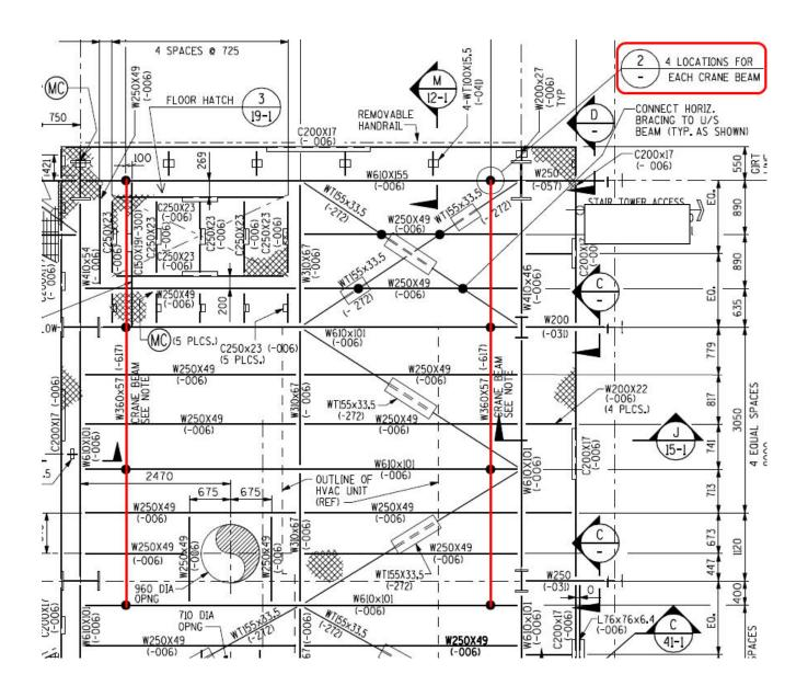
7.5 Tonne Underhung Crane Runway Beam Plan
