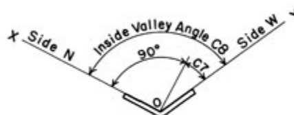
VALLEY CORNER ANGLE (Section normal to Valley)
